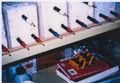
**SPECIMENS PREPARATION ACCORDING TO ASTM G109 SPECIFICATION**
