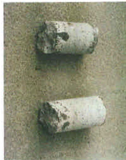
Figure 7 – Small diameter cores after pull-off test (failure through old concrete).
